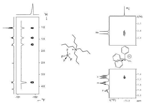
**Fig. 6**  $^{1}\text{H},^{19}\text{F}$  HOESY spectra of 2 mmol solutions of NBu<sub>4</sub>(BF<sub>4</sub>), **5**, (left, THF) and MePPh<sub>3</sub>(PF<sub>6</sub>), **6** (right, CD<sub>2</sub>Cl<sub>2</sub>).
