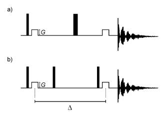
**Fig. 1** Typical pulse sequences for the PGSE experiments: (a) the Stejskal-Tanner experiment; (b) the Stejskal-Tanner experiment, modified via substitution of two 90° pulses for a single 180° pulse.
