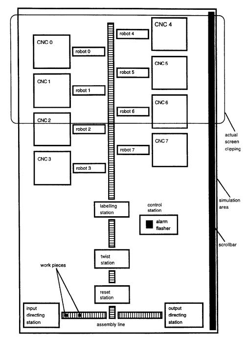
Fig. 2. The schematic view of the whole plant simulator. The rectangle shows the actual screen output that each operator can see at any given time.
