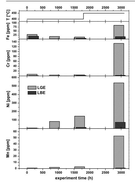
**Fig. 2.** The mass concentration of Fe, Cr, Ni and Mn in ppm found in LGE and LBE as a function of accumulated experiment time. In the upper section of the graph the operating temperature is shown, where the temperature offset represents a maintenance break for both loops.
