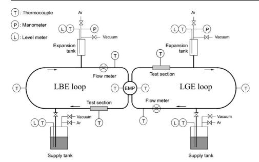
**Fig. 1.** Schematic layout of the twin-loop.
