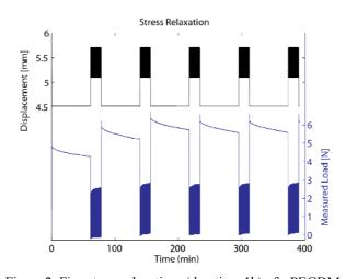
Figure 2: Five stress relaxations (duration: 1h) of a PEGDM sample-gel combined with cyclic testing (filled areas, duration: 17min, number of cycles: 1000)
