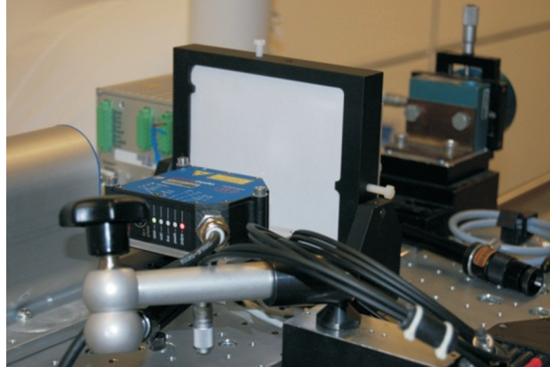
Fig. 3. Target KaH on trolley (center); triangulation sensor temporarily set up for checking target adjustment (foreground).
