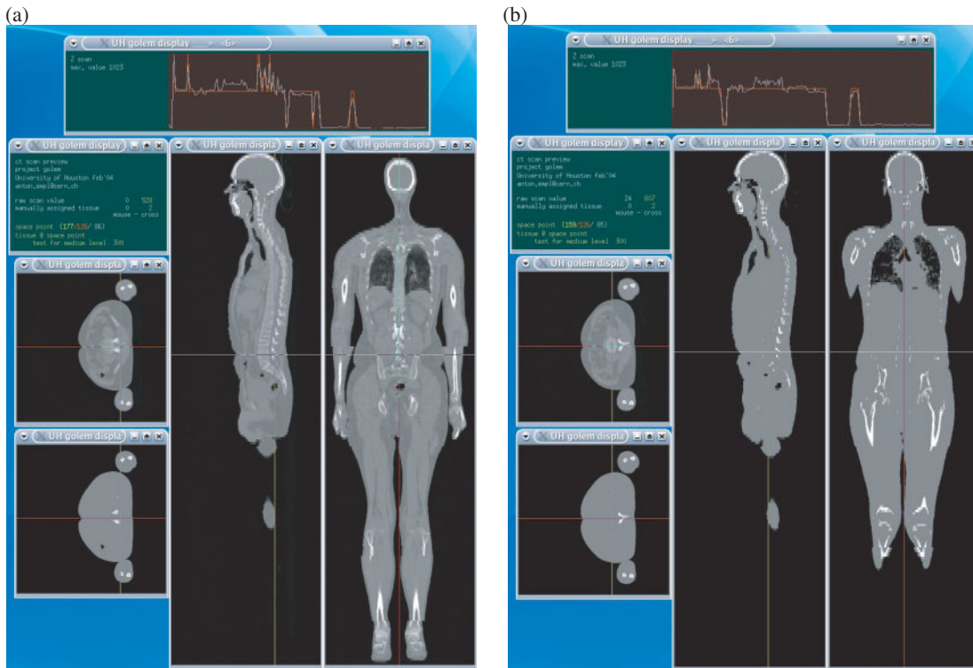
Figure 1. Screen shots are presented of the software tool developed to assess the performance of the tissue assignment algorithm. (a) A slice from the ‘Golem’ CT-scan, where the raw density values are displayed on a linear brightness scale as pixels. (b) The result of filtering this image with the simple threshold algorithm. Note the histogram tool that displays the raw data across the slice and the values from the algorithm superimposed.
