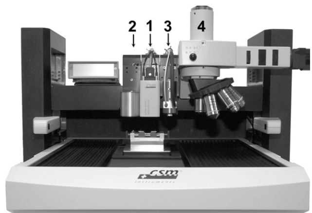
FIG. 1. The UNHT mounted on the OPX platform. The configuration includes (1) Ultra Nanoindentation measurement head, (2) Nanoindentation measurement head, (3) AFM microscope, and (4) optical microscope with camera.
