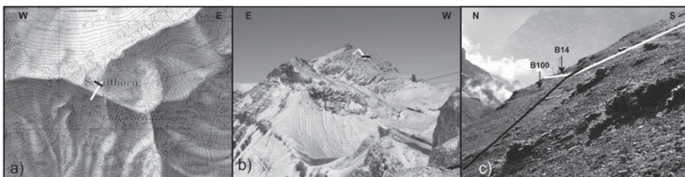
Figure 1 (a) Map (PK25, © Swisstopo 2007) and (b and c) photographs of the Schilthorn field site with location of the automated electrical resistivity tomography (A-ERT) profile (black), boreholes (B14 and B100) and the additional ERT line across the Schilthorn ridge (white).
