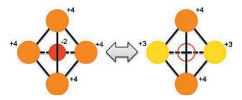
Figure 1. Simplified schematic representation of the charge redistribution in CeO<sub>2</sub> upon the occurrence of an oxygen vacancy. Adapted with permission from ref.<sup>[16]</sup>
