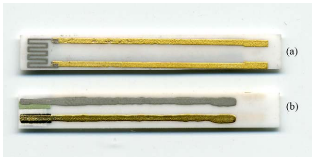
Fig. 8. Single-chamber fuel cell supported on alumina substrate: (a) platinum heater and (b) SCFC with screen-printed YSZ (4 mm × 4 mm), NiO-YSZ and LSM electrodes (4 mm × 1 mm) and gold and platinum collectors.
