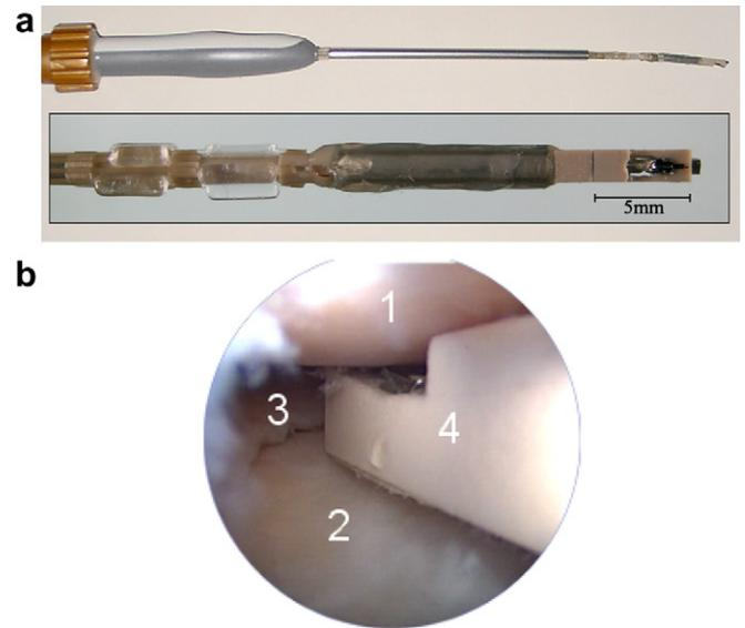
Fig. 3. (a) Arthroscopic AFM for measuring in a minimal invasive approach the elasticity of articular cartilage in the knee joint. (b) Tool tip inside a knee joint as seen through an optical arthroscope. (1) Cartilage of the femoral condyle, (2) cartilage of the tibial plateau, (3) meniscus and (4) AFM-tip measuring the surface of the cartilage of the femoral condyle.
