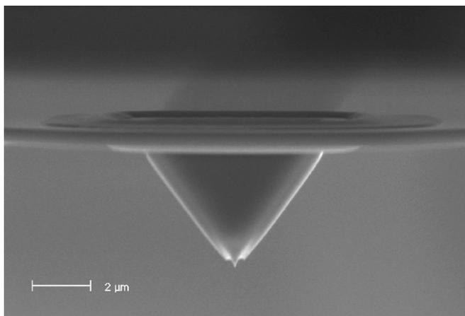
Fig. 1. Conductive cantilever with electrical insulation for operation in physiological buffer solution or for electrochemical experiments. Only the metal tip apex reaches about 100 nm out of the  $\text{SiO}_2$  insulation.
