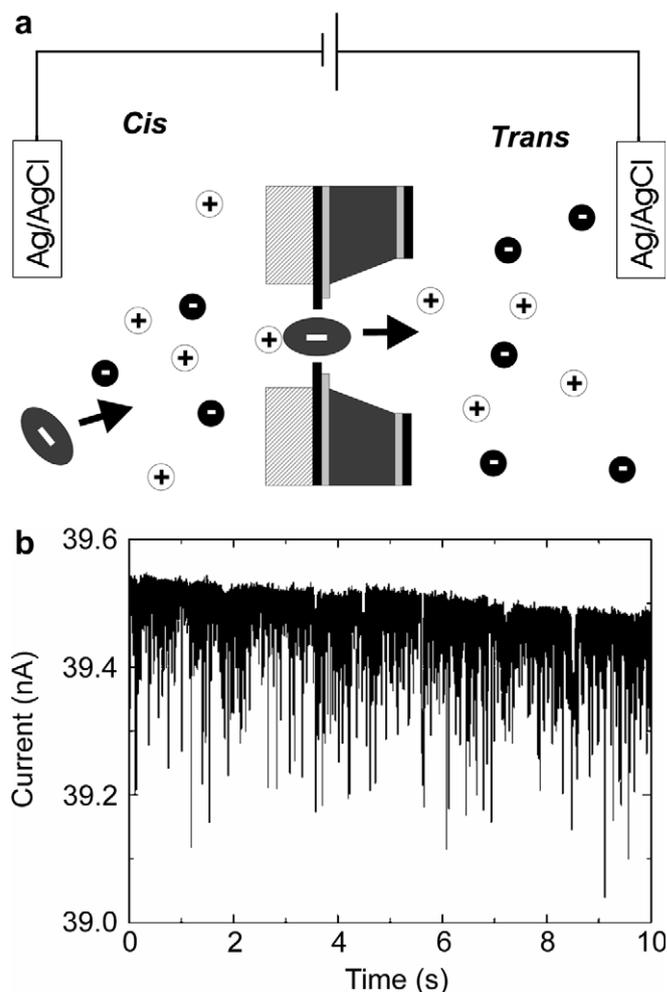
Fig. 2. (a) Concept of nanopore measurements. The ionic current through a small orifice is temporarily reduced when a molecule is translocated, giving rise to the current drops seen on the right hand side (b).
