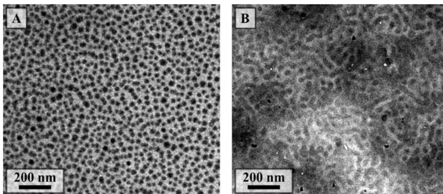
**Figure 2.** Representative TEM micrographs of dry PS-*block*-PNIPAM-*block*-PS triblock copolymer thin films with spherical and bicontinuous morphology: (A) sample PN77.118K with 77 wt % PNIPAM and (B) sample PN61.106K with 61 wt % PNIPAM.
