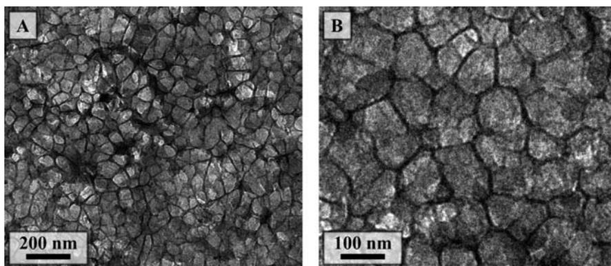
**Figure 5.** (A) Cryo-TEM images of sample PN61.106K having bicontinuous morphology. Sample is vitrified from the swollen hydrogel state ( $T = 5$  °C) followed by in situ freeze-drying at  $-80$  °C. (B) Higher magnification clearly reveals the continuous plastically deformed polystyrene network with 3-fold and 4-fold symmetry in the junction points.
