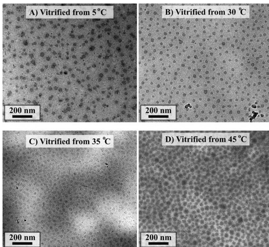
**Figure 3.** Cryo-TEM micrographs of PS-*block*-PNIPAM-*block*-PS block copolymer hydrogel sample PN77.118K xposed to water: (A) vitrified from 5 °C and 100% humidity; (B) vitrified from 30 °C and 100% humidity; (C) vitrified from 35 °C and 100% humidity; (D) vitrified from 45 °C and 100% humidity. A sharp transition in the distance between the polystyrene spheres occurs between 30 and 35 °C.
