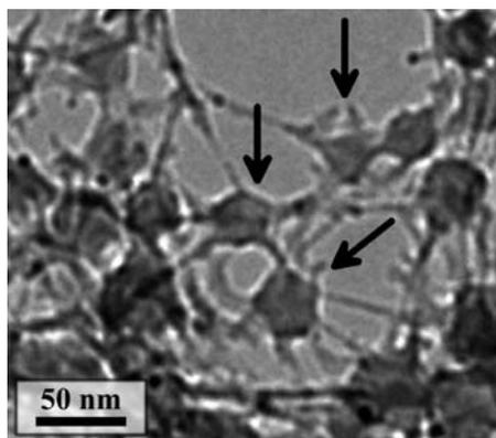
**Figure 6.** High-magnification freeze-dried cryo-TEM micrograph of the PN77.118K sample with spherical morphology. Sample is vitrified from the swollen hydrogel state ( $T = 5$  °C). Arrows highlight the polystyrene spheres which have transformed into polyhedrons (with pentagonal or triangular projections in the TEM image) by extensive plastic deformation.
