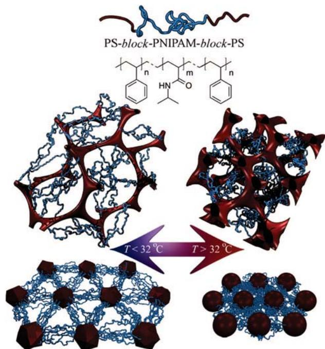
**Figure 1.** Chemical structure of polystyrene-*block*-poly(*N*-isopropylacrylamide)-*block*-polystyrene triblock copolymer and a schematic illustration of temperature-induced conformation transition of aqueous hydrogel having self-assembled morphologies with spherical or “gyroid” PS domains. In both cases, PS domains act as physical cross-links for the hydrogel.
