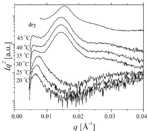
**Figure 7.** Small-angle X-ray scattering diffractograms of PN77.118K. Dry bulk sample at room temperature and for the hydrogel–water mixture collected after swelling upon heating from 20 to 45 °C measuring every 5 °C. Data show a very sharp structural transition at the PNIPAM coil-to-globule transition temperature, which occurs between 30 and 35 °C.
