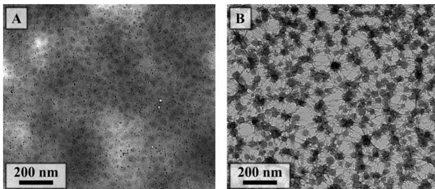
**Figure 4.** In-situ freeze-dried cryo-TEM micrograph of PS-*block*-PNIPAM-*block*-PS block copolymer hydrogel sample PN77.118K exposed to water: (A) sample vitrified from 45 °C; (B) sample vitrified from 5 °C.
