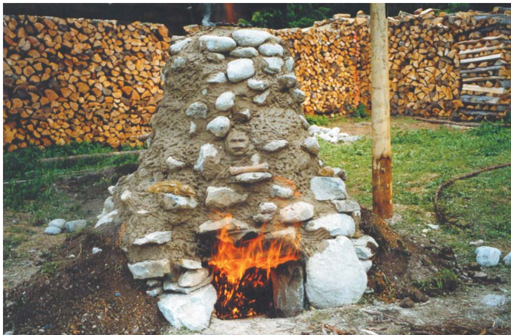
Figure 1 The experimental shaft furnace with a height about 2 m.
